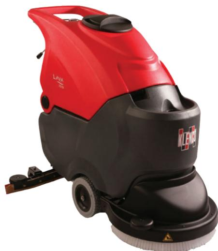
**LAVA 501B & C** are workhorses for small to mid sized commercial applications. Thorough cleaning is achieved with up to 30kg brush down pressure, while the floating V-type squeegee effectively dries tiled and uneven floors. Hands-free latching/ release of brush or pad holder and tool-free change of squeegee blades all add up to simple maintenance and maximum productivity.
